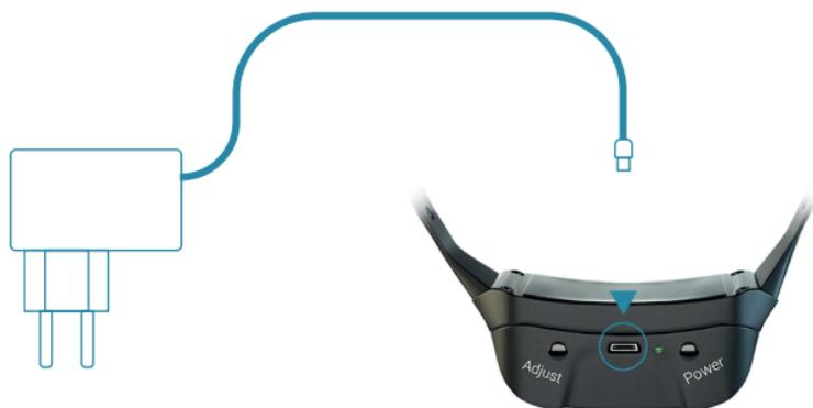
With the aid of the charging cable, fully charge the Antibark Spray Trainer Advance until the LED is permanently lit green. As long as the LED is red and green, the device is not fully charged.
