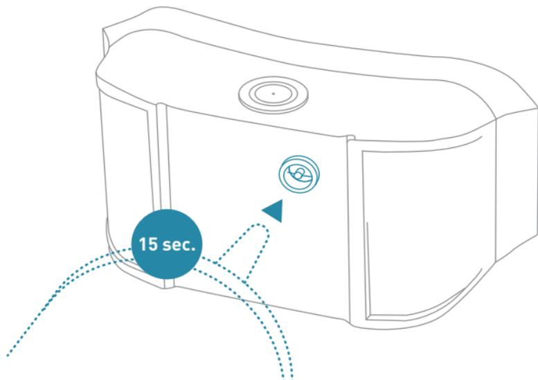
The Antibark Spray Trainer Advance must be switched off to fill with spray. For this purpose, the filling nozzle must be placed vertically on the filling valve. When the filling nozzle is properly positioned, gently press and fill the trainer for 15 seconds.
