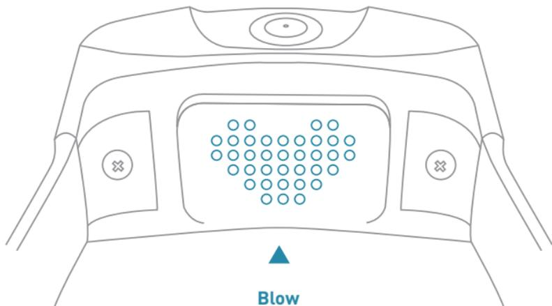
Check whether the battery is charge and the trainer is switched on. Subsequently, blow from the back against the sensor, so that the trainer issues a spray signal.
