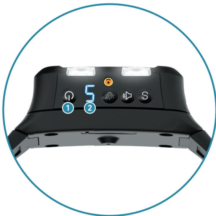
To switch off the Modular Spray Trainer, the switch-off button must be pressed for several seconds until you hear a beep.
